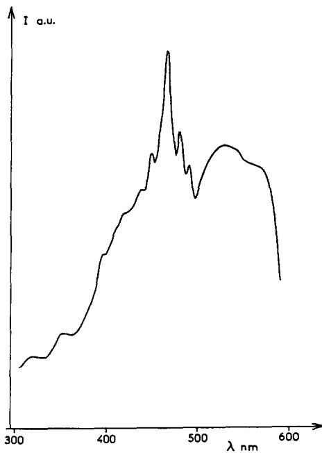
Fig. 6b. Excitation spectrum of orange-red compound 2; analysis at 600 nm; maximum at 466 nm.
